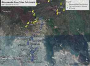
Catchment area map of Village Tank, Bampewada, prepared by using GPS
