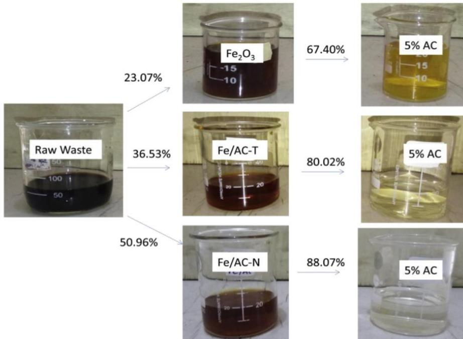
**Color reduction of waste water after proposed wet oxidative pre-treatment over heterogeneous iron catalyst and adsorption on activated carbon**
